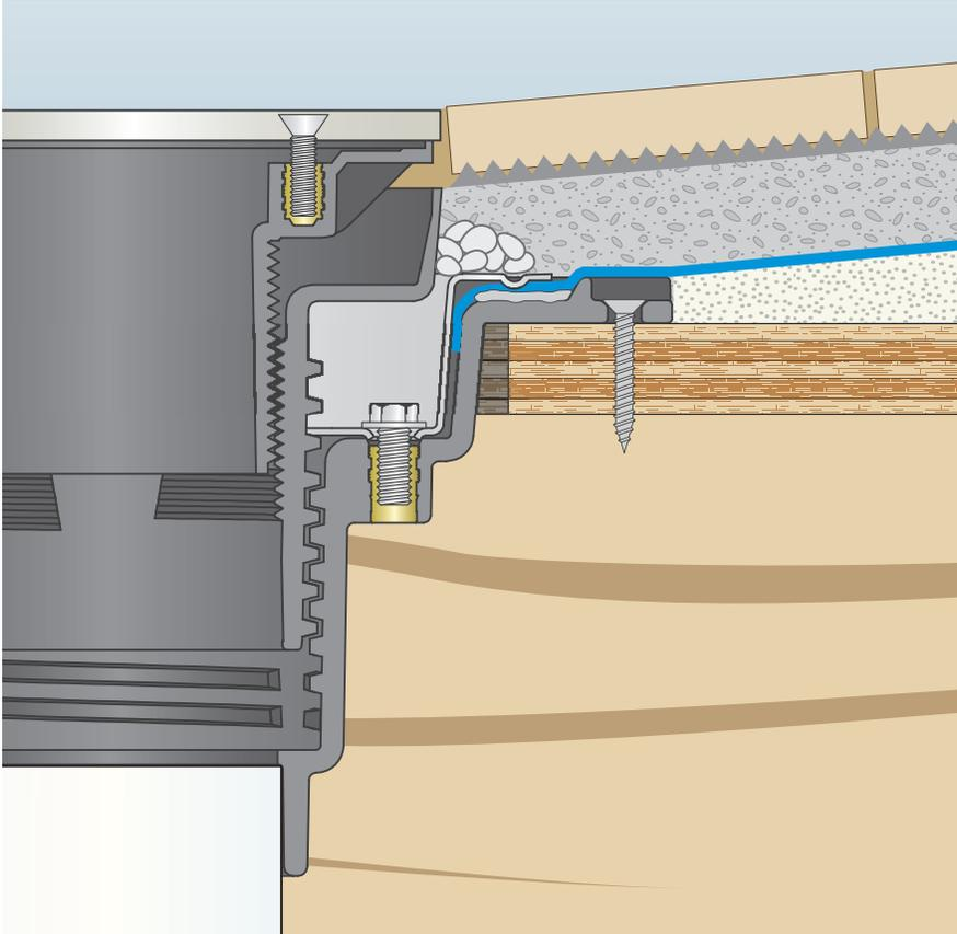
In a traditional shower pan application with sheet pan liner, the Coring Sleeve allows for a faster, easier installation of the secondary mortar bed.
