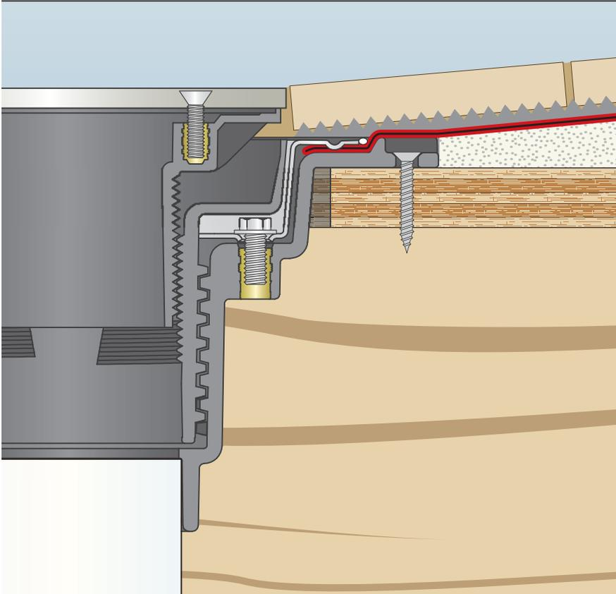
For shower floors using liquid waterproofing or a fabric-bonded sheet liner, the stainless steel clamping collar is fastened on the inside recess of the drain body.
