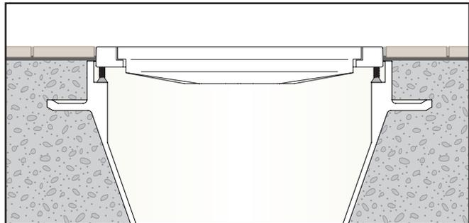
Install the adjustable frame and level with the new/added flooring. The separate frame allows the grate to be removed and replaced as needed.
