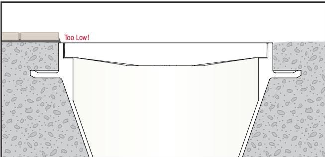
Even when fixture is installed flush/level with slab, adding tile or other flooring later can leave the grate too low, creating a trip hazard.
