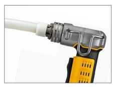
3. Using expander tool, expand sleeve fully. If using a manual tool, expand slowly and repeat expansions, rotating expander 1/8-turn between expansions. Forcing the tube onto the expansion head and/or expanding too quickly can damage the tubing and sleeve, and require rework.
