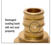
Damaged, cut or grooved barb on fitting.
